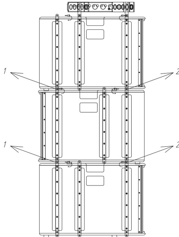
**Fig.31.** X-215W Flying, three units in cardioid configuration
