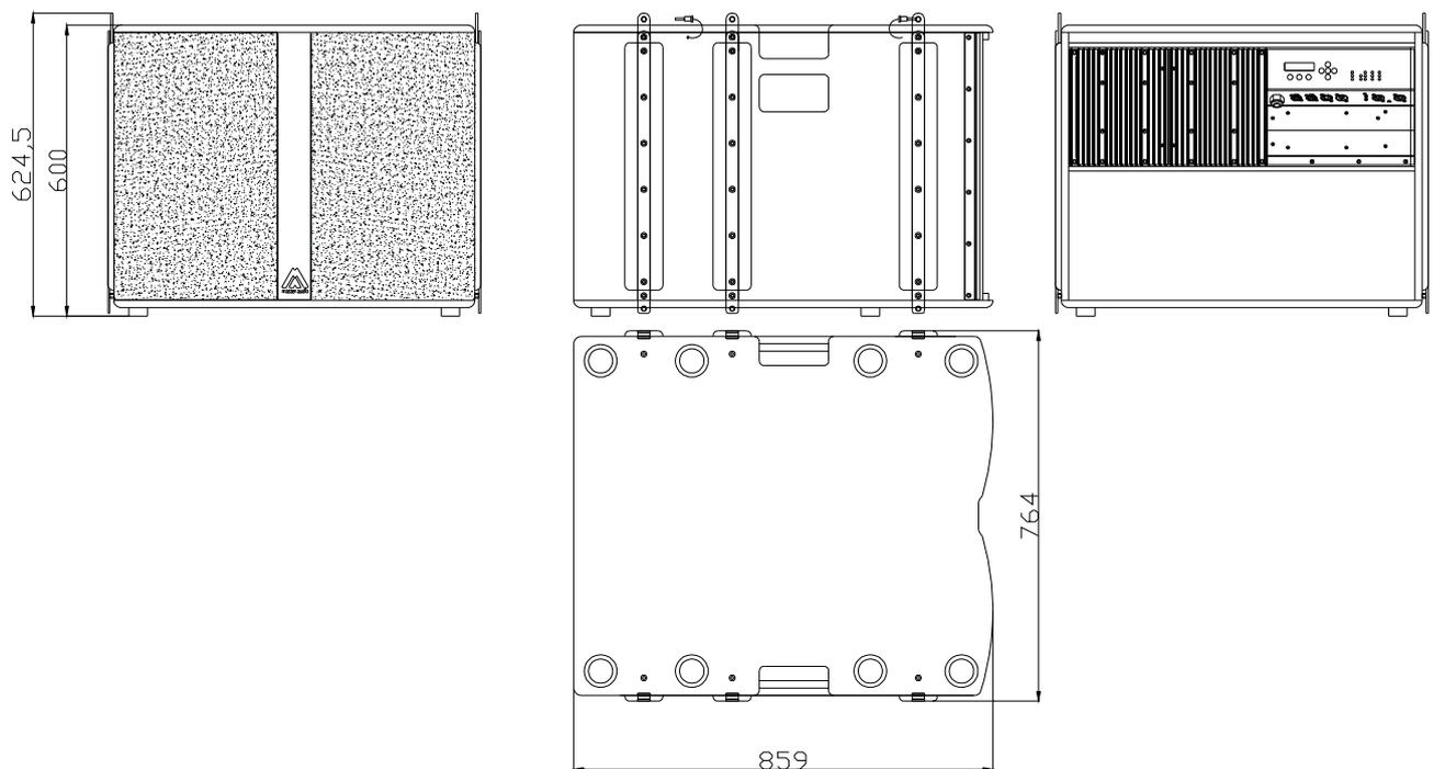
**Fig.11.** X-215W cabinet. External dimensions
