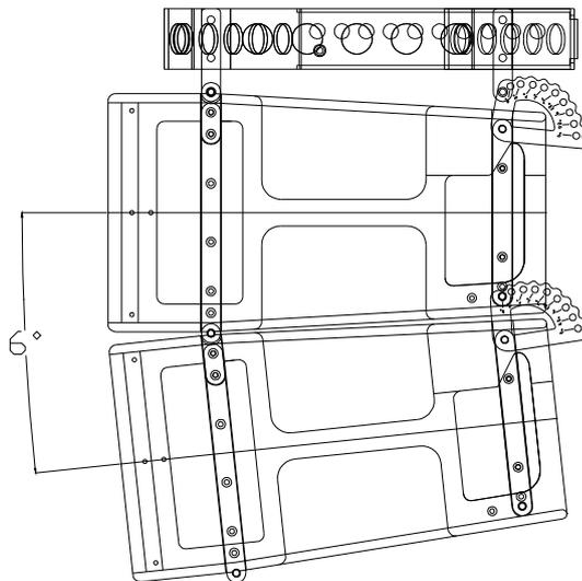
**Fig.4.** Tilt angle between cabinets ( $6^\circ$  maximum)
