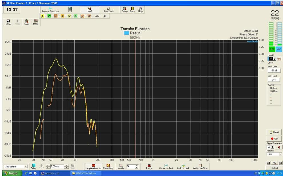
**Fig.22b.** X215W total back energy rejection. Yellow curve without central cardioid subwoofer; orange curve adding central cardioid subwoofer.
