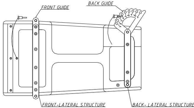
**Fig.24.** Flying hardware (lateral view)
