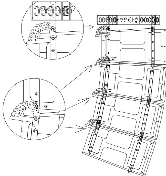
**Fig.29.** X-210 Flying. 6° Curved Line Array (Cabinet 1 Back Guide = SW)
