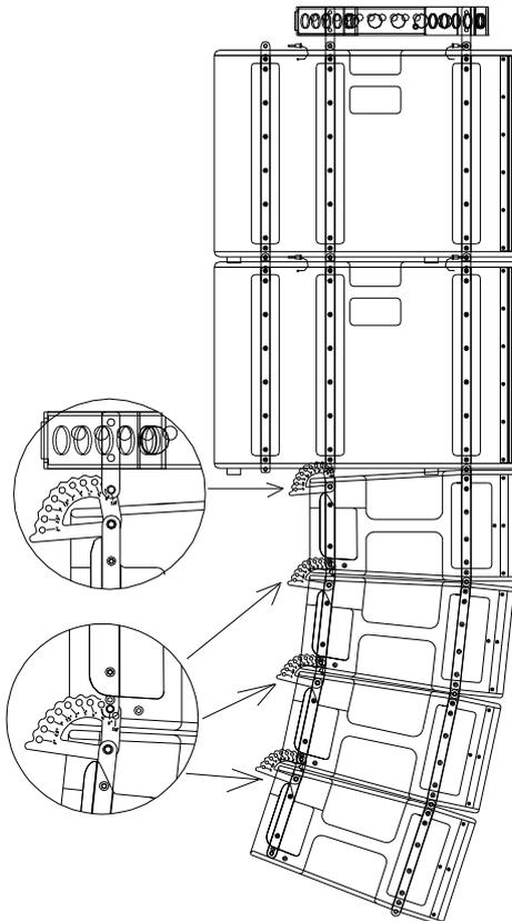
**Fig.33.** X-210 + X-215W Flying, curved Line Array
