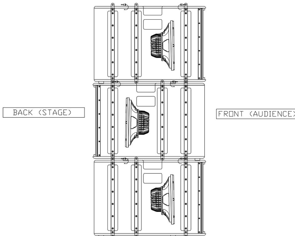
**Fig.19.** Cardioid configuration for X-215W subwoofer
