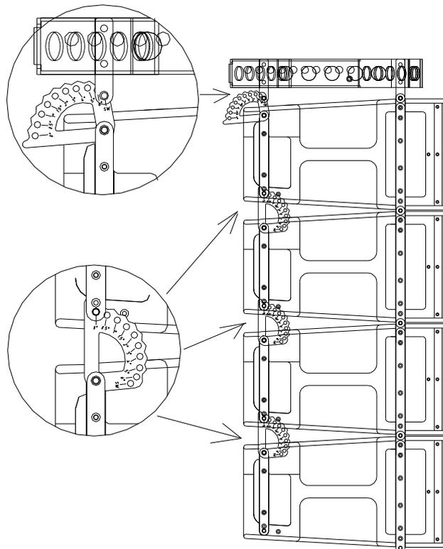
**Fig.28.** X-210 Flying. Flat Line Array (Cabinet 1 Back Guide = SW)
