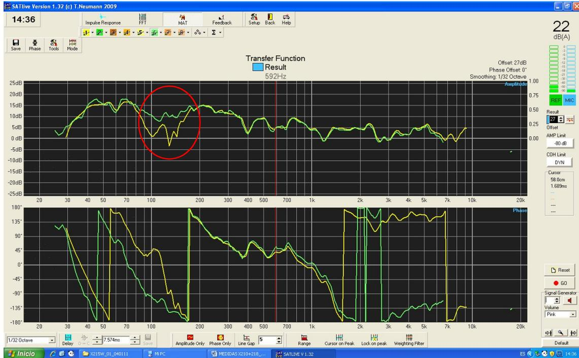
**Fig.36.** Magnitude and phase response of the complete aligned system (with delay), green curve
